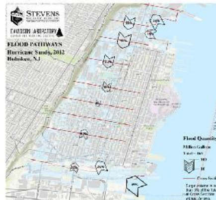
Figure 3-4: Flood Pathways, Hoboken, NJ. In partnership with the State, Stevens Institute of Technology is creating and testing models to understand flood pathways. These models can provide information on local risks and can inform the selection of appropriate risk reduction measures and characterize the benefits and efficacy of different options. The State's assessment of flood pathways in Hoboken, New Jersey (pictured), for example, highlights the State's ongoing work to identify effective strategies for densely populated urban settings.
